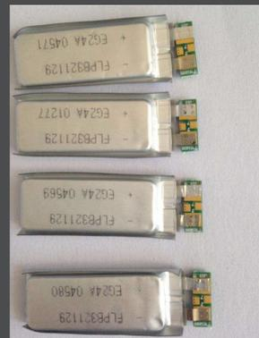
While welding is the preferred method of connection, it is important to note that welding directly to a battery may cause leakage, venting, or in extreme cases, explosion and/or fire. Therefore, only interconnect the cells by spot welding to the flat strip (tab) terminations and perform spot welding behind safety shields.
